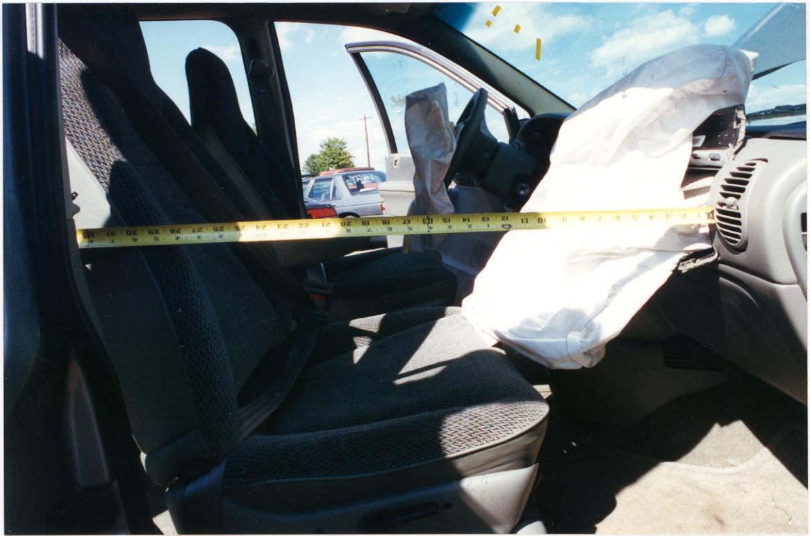
83. Longitudinal measurement of the position of the seat relative to the instrument panel.
